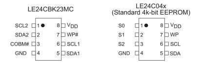
The Pin 3 (slave pin: S2) function of a regular 4K-bit EEPROM product is assigned to the COBM# pin of the LE24CBK23MC.
