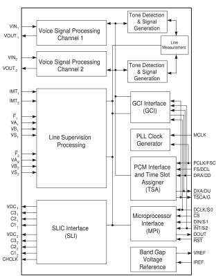
Figure 1. Le78D11 VoSLAC Device Block Diagram
