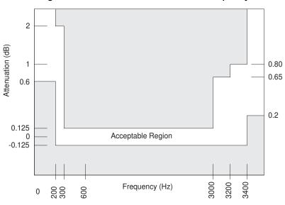
Figure 2. Transmit Path Attenuation vs. Frequency
