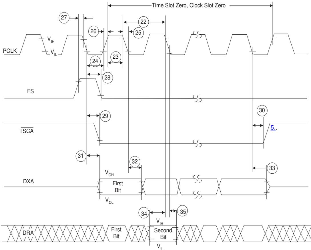
Figure 14. PCM Highway Timing for XE = 1 (Transmit on Positive PCLK Edge)
