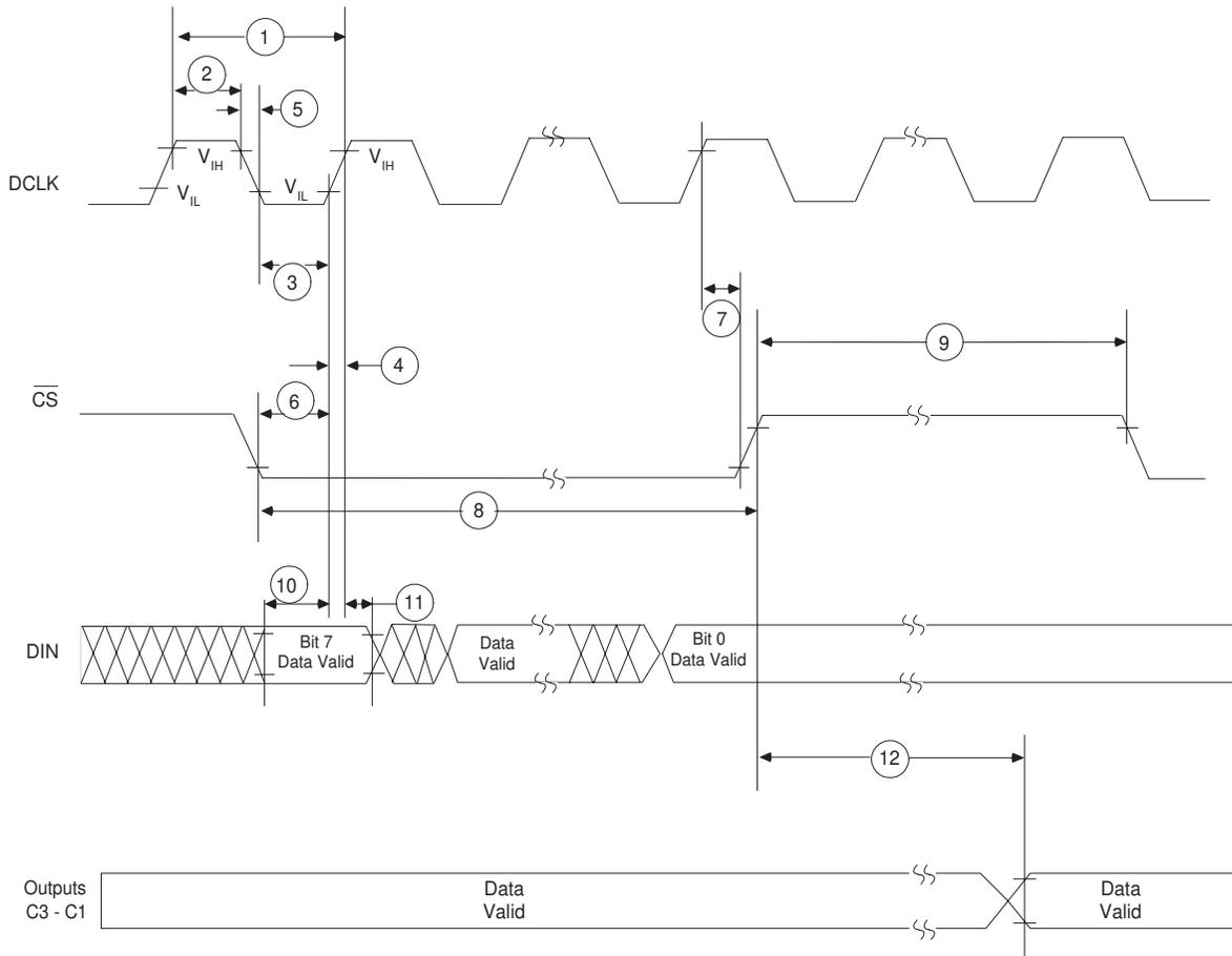
Figure 12. Microprocessor Interface (Output Mode)
