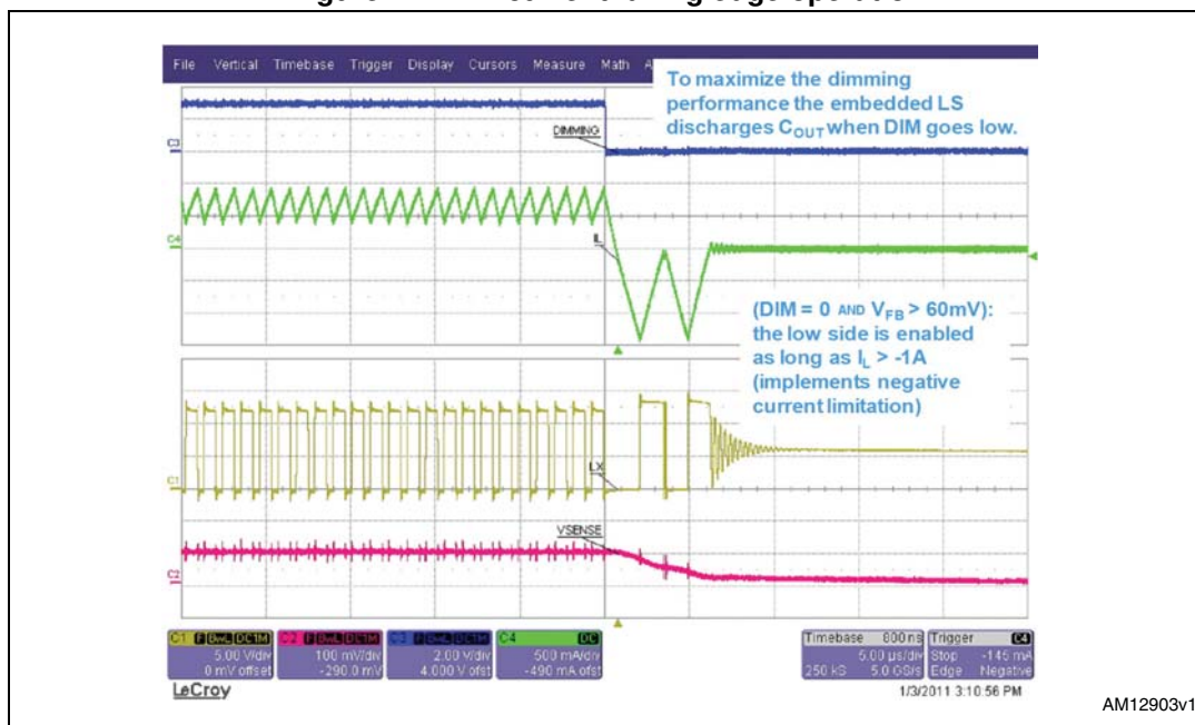
Figure 12. LED current falling edge operation
