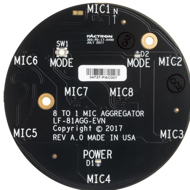
Figure 6.2. 8 to 1 Mic Aggregator Board (Daughter Board)
