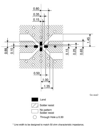
Depending on PCB material and thickness.
