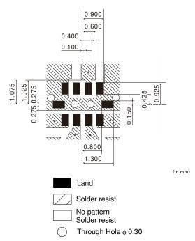
$\boxtimes\square$  Line width to be designed to match 50  $\Omega$  -characteristic impedance, depending on PCB material and thickness.
