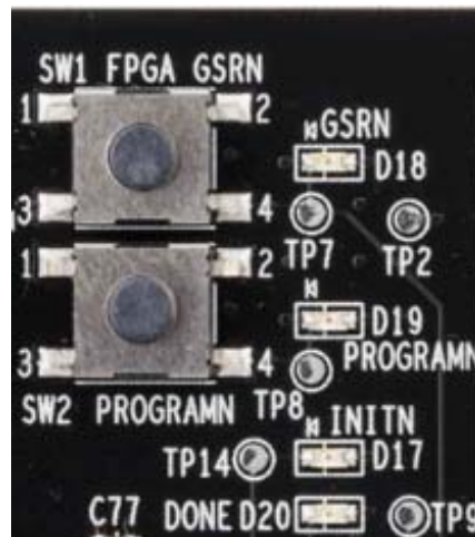
Figure 3. ECP5 Status LEDs and Push-button Controls
