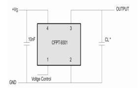
\* Load 15pF (HCMOS), inclusive of probe and jig capacitance
