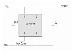
\* Load 15pF (HCMOS), inclusive of probe and jig capacitance
