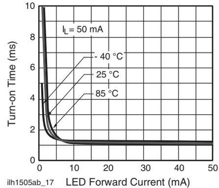
Fig. 18 - Turn-on Time vs. LED Current
