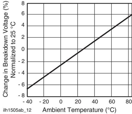
Fig. 13 - Switch Breakdown Voltage vs. Temperature
