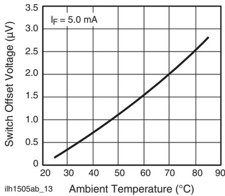
Fig. 14 - Switch Offset Voltage vs. Temperature
