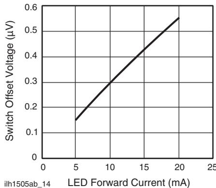
Fig. 15 - Switch Offset Voltage vs. LED Current
