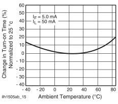
Fig. 16 - Turn-on Time vs. Temperature
