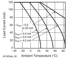
Fig. 1 - Recommended Operating Conditions
