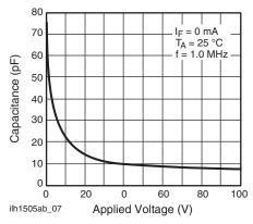
Fig. 8 - Switch Capacitance vs. Applied Voltage
