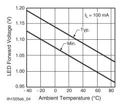
Fig. 5 - LED Dropout Voltage vs. Temperature
