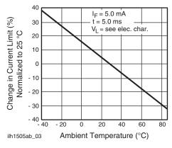
Fig. 4 - Current Limit vs. Temperature
