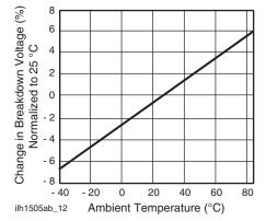
Fig. 13 - Switch Breakdown Voltage vs. Temperature
