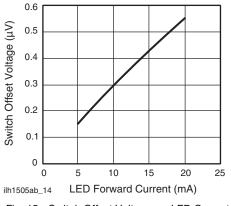
Fig. 15 - Switch Offset Voltage vs. LED Current
