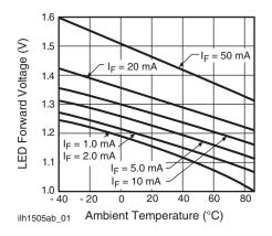
Fig. 2 - LED Voltage vs. Temperature
