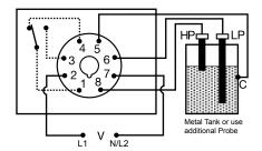
HP = HIGH LEVEL PROBE LP = LOW LEVEL PROBE C = PROBE COMMON V = VOLTAGE
