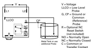
Relay contacts are isolated. Connect common to conductive tank. Additional probe is necessary for non-conductive or insulated tanks.
