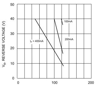
T<sub>A</sub>, AMBIENT TEMPERATURE (°C) Fig. 3 Blocking Voltage Derating Curves
