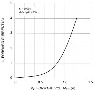
Fig. 1 Typical Forward Characteristics
