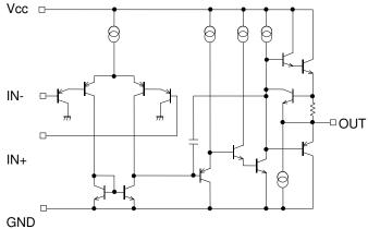
Fig.97 Circuit Diagram (each Op-Amp)
