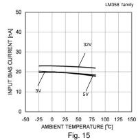
Input Bias Current – Ambient Temperature (Vicm=0[V], VOUT=1.4[V])
