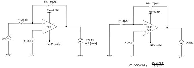
Fig.101 Measurement Circuit 3
