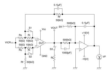
Fig.98 Measurement Circuit 1 (each Op-Amp)
