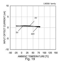
$\begin{array}{c} \text{Input Offset Current} - \text{Ambient Temperature} \\ (\text{Vicm=0[V]}, \text{VOUT=1.4[V]}) \end{array}$
