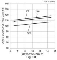
Large Signal Voltage Gain – Supply Voltage  $(RL=2[k\Omega])$
