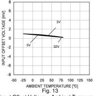
Input Offset Voltage – Ambient Temperature (Vicm=0[V], VOUT=1.4[V])
