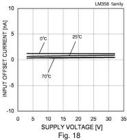
Input Offset Current – Supply Voltage (Vicm=0[V],VOUT=1.4[V])
