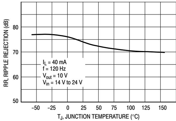
**Figure 7. Ripple Rejection**
