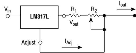
$$I_{outmax} = \left( \frac{V_{ref}}{R_1} \right) + I_{Adj} \cong \frac{1.25 \text{ V}}{R_1}$$
