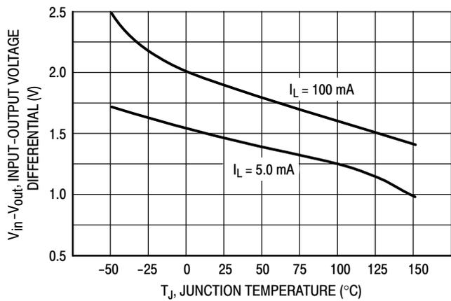
**Figure 9. Dropout Voltage**
