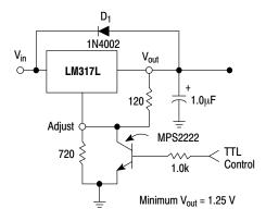
D<sub>1</sub> protects the device during an input short circuit.
