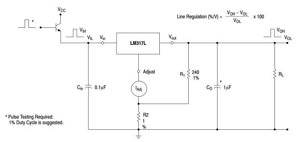
Figure 2. Line Regulation and  $\Delta I_{\mbox{Adj}}/\mbox{Line}$  Test Circuit
