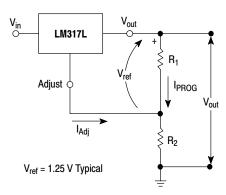
Figure 18. Basic Circuit Configuration
