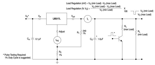
Figure 3. Load Regulation and  $\Delta I_{\mbox{\scriptsize Adj}}/\mbox{\scriptsize Load}$  Test Circuit
