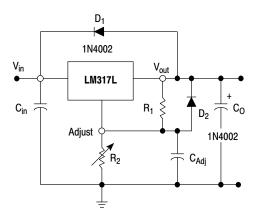
Figure 19. Voltage Regulator with Protection Diodes
