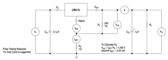
Figure 4. Standard Test Circuit
