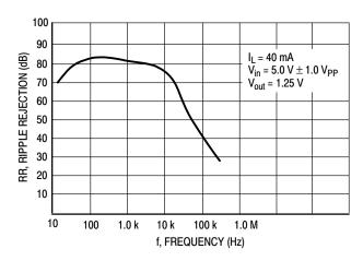
Figure 11. Ripple Rejection versus Frequency
