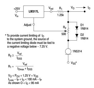
Figure 20. Adjustable Current Limiter
