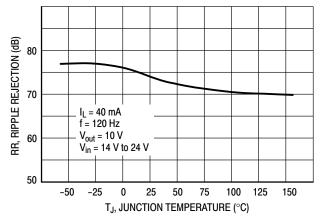
Figure 7. Ripple Rejection
