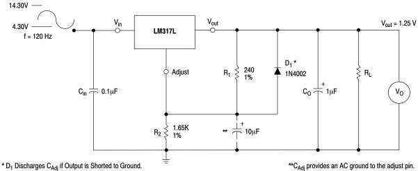
Figure 5. Ripple Rejection Test Circuit
