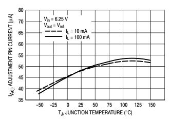
Figure 13. Adjustment Pin Current
