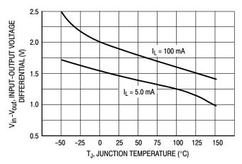
Figure 9. Dropout Voltage
