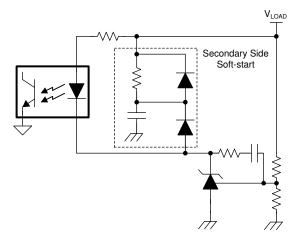
Figure 9-9. Secondary-Side Soft Start in Flyback
