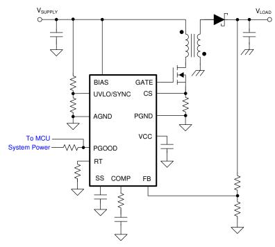
Figure 10-12. Typical Non-Isolated Flyback
