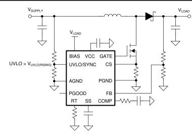
Figure 9-6. Decrease the Minimum Operating Voltage After Start-Up
