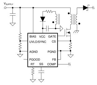
Figure 9-7. External VCC Supply (BIAS ≥ VCC)
