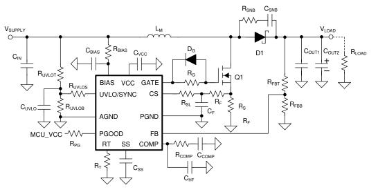
Figure 10-1. Typical Boost Converter Circuit With Optional Components
