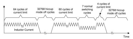
Figure 9-20. Hiccup Mode Overload Protection
