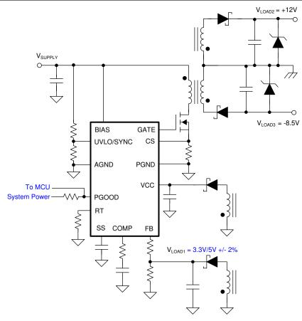
Figure 10-11. Primary-Side Regulated Multiple-Output Isolated Flyback
