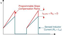
Figure 9-18. Slope Compensation Ramp (a) at PWM Comparator Input
