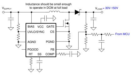
Figure 10-7. LIDAR Bias Supply 1
