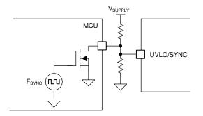
Figure 9-11. UVLO, Shutdown, and Clock Synchronization
