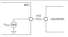
Figure 9-15. Shutdown and Clock Synchronization
