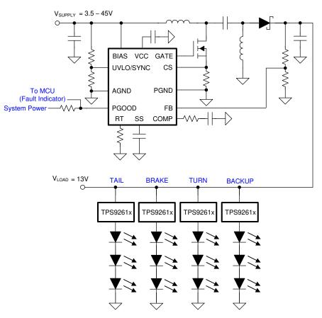
Figure 10-14. Dual-Stage Automotive Rear-Lights LED Driver
