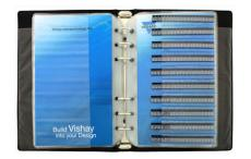
Files contain lengths of blister tape, each holding 20 resistors. The kit contains every fourth value of the E 96-series. Parts are sorted in the ascending order of its resistance value and appropriately marked.
