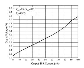
**Output Voltage vs. Output Sink Current**
