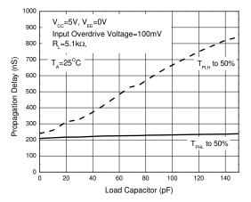
Propagation Delay vs. Load Capacitors
