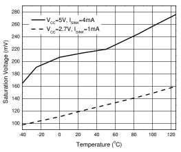
Saturation Voltage vs. Temperature
