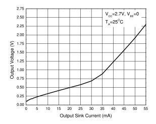
**Output Voltage vs. Output Sink Current**
