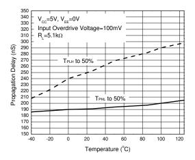
**Propagation Delay vs. Temperature**
