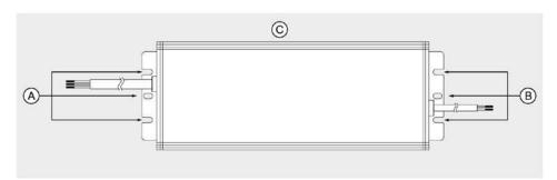
Fig. 3 Mounting Hole Locations
