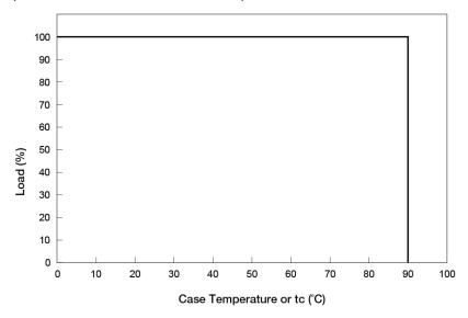
The LED Driver can support 100% rated load for case hot spot surface temperatures of less than 90°C.
