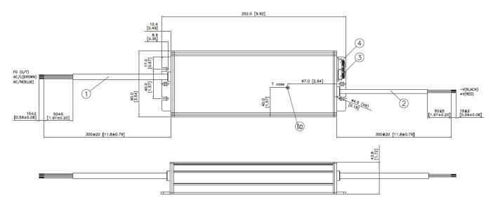
LNE-□V320WB□A (IP67 without dimming cable & potentiometers)
