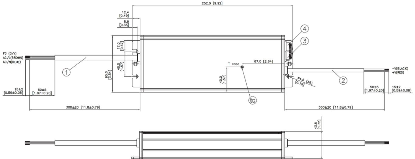
LNE-□V320WB□A (IP67 without dimming cable & potentiometers)
