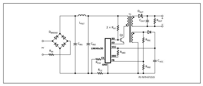
Figure 10. Typical Universal Input, 10 W Charger.
