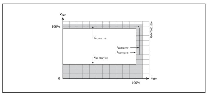
Figure 11. Typical CV/CC Output Characteristic Achieved.
