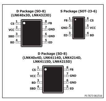
Figure 6. Pin Configuration.
