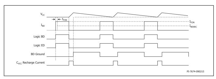
Figure 9b. Base Drive Waveforms – Easy Start mode of Operation.
