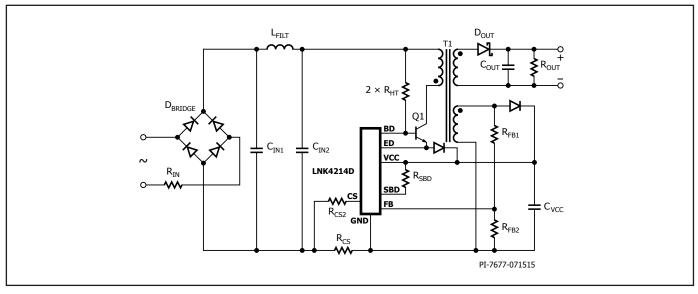
Figure 14. Typical Universal Input, 12 W Adapter.
