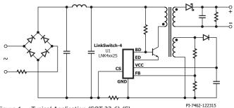
Figure 1. Typical Application (SOT-23-6) (S).
