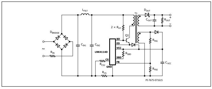
Figure 12. Typical Universal Input, 12 W Adapter.
