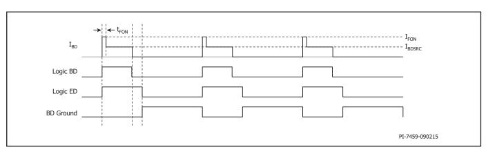
Figure 9. Base Drive Waveforms.
