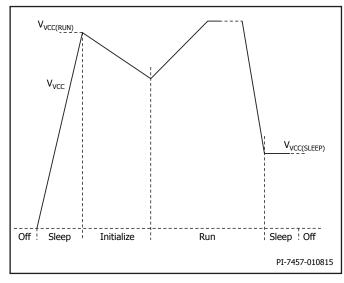
Figure 7. VCC Waveforms.
