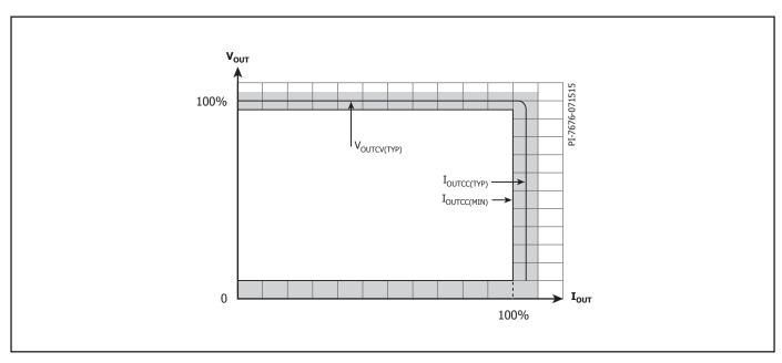
Figure 13. Typical LNK4114D and LNK4115D CV/CC Output Characteristic Achieved.
