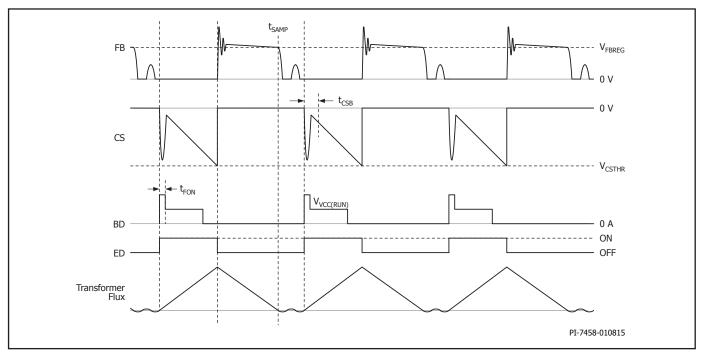
Figure 8. Typical Waveforms at the Feedback and Primary Current Sense Inputs.
