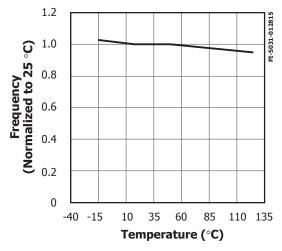
Figure 5. Output Frequency vs. Temperature.
