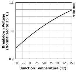
Figure 7. Breakdown vs. Temperature.
