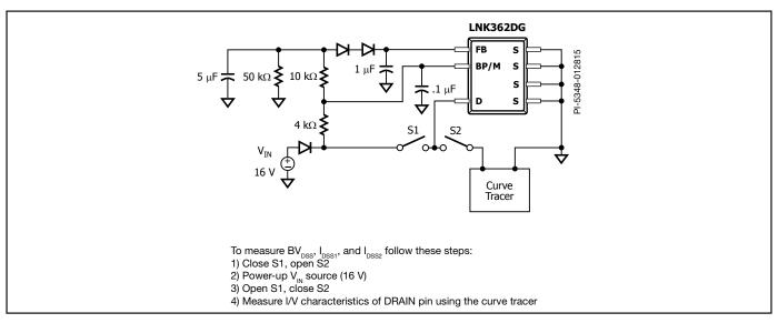
Figure 11. Test Set-up for Leakage and Breakdown Tests.
