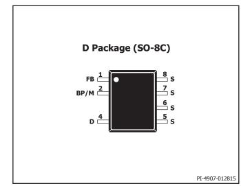
Figure 4. Pin Configuration.
