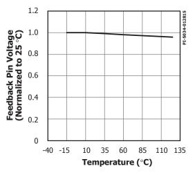
Figure 6. FEEDBACK Pin Voltage vs. Temperature
