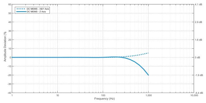
Note that the MEMS accelerometer has a DC response (can measure down to 0 hertz). The plot only goes to 1 Hz because it is on a logarithmic scale. The accelerometer data was generated with the sample rate at 3.2 kHz, and the unit taped to the mounting fixture.
