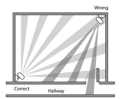
When placing the sensor in a room, do not place where the sensor is aimed out through a door. The sensor can detect hallway traffic, forcing lights-on.
