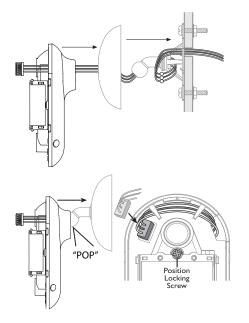
2. Connect building wiring harness with wire nuts. Snap bracket cover in place to conceal wiring and bracket. Feed wiring harness through the back of the sensor body and out exit slot.
