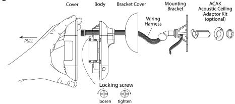
1. Insert wiring through bracket legs. Secure bracket to wall or ceiling. For ACAK Installation see page 2.
