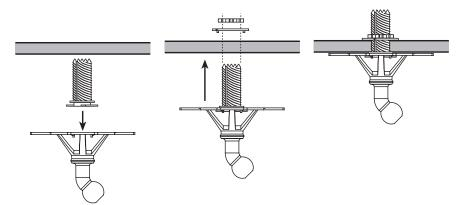
Insert ACAK into mounting bracket and twist clockwise 90° to lock into place. Screw bracket and self-cutting AKAC into ceiling tile and secure with washer and nut.
