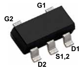
5-Lead SOT-23 (Top View)
