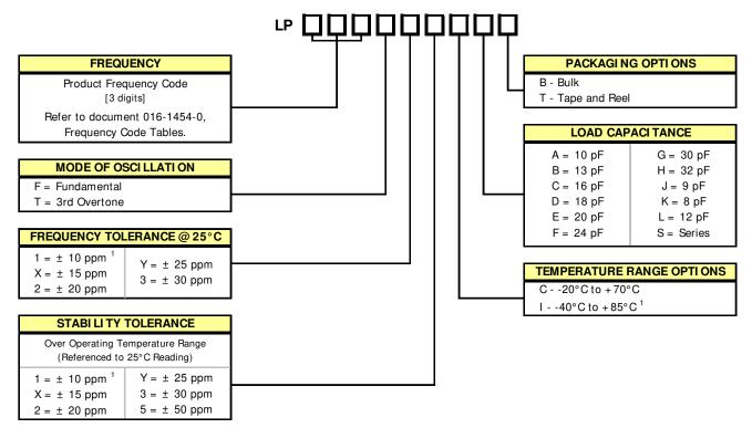
1] Check factory availability for "111" Tolerance/Stability/Temperature combination.
