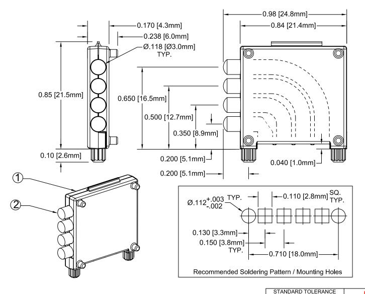
UNLESS OTHERWISE SPECIFIED )  $X^{\circ} \pm 1^{\circ}$ TEL: (949) 951-8808 FAX: (949) 951-3974 XX. ± .02 QUAD-LEVEL LIGHT PIPE TITLE: XXX ± .010 ASSEMBLY, EXTENDED LENS DESIGNED: PART NO: LP4-EP 08/26/02 Michael Chen CHECKED: CAGE CODE: 32559 SHEET# 1 OF 1 S. Irving 08/26/02 CAD GENERATED DOCUMENT, DO NOT MEASURE DRAWING.
