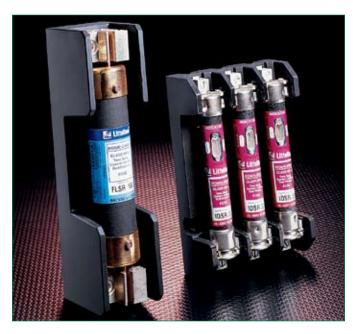
Class H and Class R fuse blocks are dimensionally the same, but Class R blocks incorporate a rejection feature, which only allows Class R fuses to be inserted.
