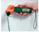
380940 400A AC/DC Watt Clamp Meter Versatile electrical test tool with
