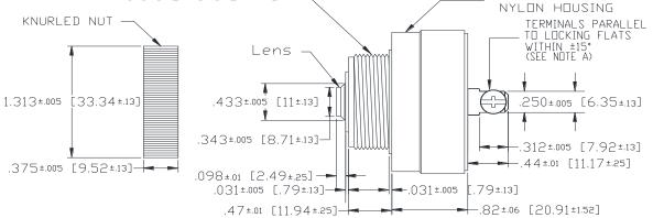
NOTE A: TERMINALS-.032 BRASS TIN PLATED, TAPPED FOR #6-32 SCREW. TWO #6-32 NI PLATED BRASS SCREWS TWO #6-32 NICKEL INCLUDED. WILL ACCEPT 1/4" QUICK CONNECT.
