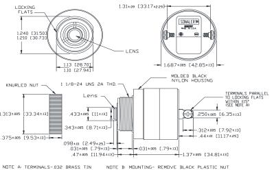
NOTE A: TERMINALS-032 BRASS TIN PLATED, TAPPED FOR #6-32 SCREW. TWO #6-32 NICKEL PLATED BRASS SCREWS INCLUDED. WILL ACCEPT 1/4' QUICK CONNECT. NOTE B: MOUNTING- REMOVE BLACK PLASTIC NUT
