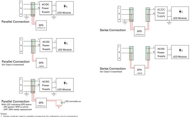
Series module used in parallel connection for indication circuit connection
