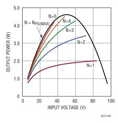
Figure 3. Output Power for 12V Output
