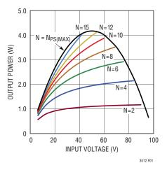
Figure 1. Output Power for 3.3V Output
