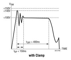
Figure 5. Maximum Voltages for SW Pin Flyback Waveform
