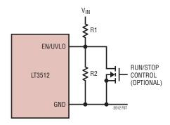
Figure 7. Undervoltage Lockout (UVLO)
