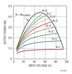
Figure 2. Output Power for 5V Output
