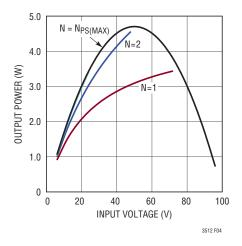
Figure 4. Output Power for 24V Output
