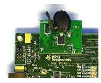
The CC2530EM, with the antenna mounted on the SMA connector, can be plugged into a SmartRF05EB. The SmartRF05EB is included in the CC2530 Development Kit [2].
