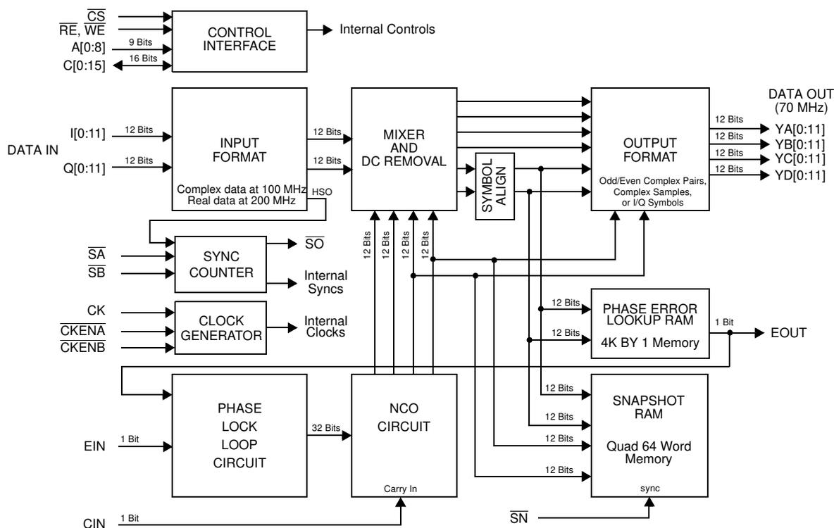
Figure 1. GC3021A BLOCK DIAGRAM
