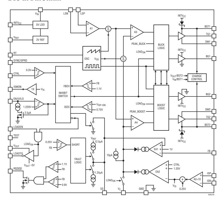
The LT8390A is a current mode DC/DC controller that can regulate output voltage, input or output current from input voltage above, below, or equal to the output voltage. The LTC proprietary peak-buck peak-boost current mode control scheme uses a single inductor current sense resistor and provides smooth transition between buck region, buck-boost region, and boost region. Its operation is best understood by referring to the Block Diagram.
