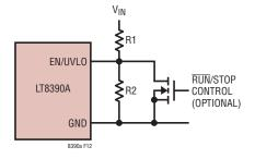
Figure 12. V<sub>IN</sub> Undervoltage Lockout (UVLO)
