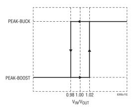
Figure 2. Current Mode vs V<sub>IN</sub>/V<sub>OUT</sub> Ratio
