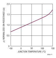
Figure 11. Normalized  $R_{DS(ON)}$  vs Temperature
