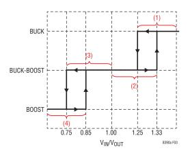
Figure 3. Operation Region vs V<sub>IN</sub>/V<sub>OUT</sub> Ratio
