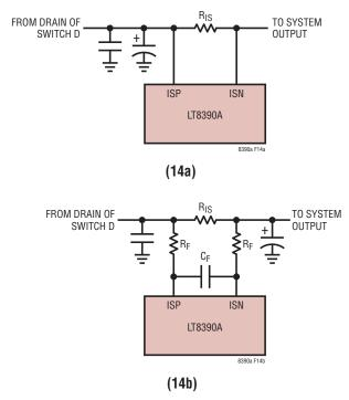
Figure 14. Programming Output Current Limit
