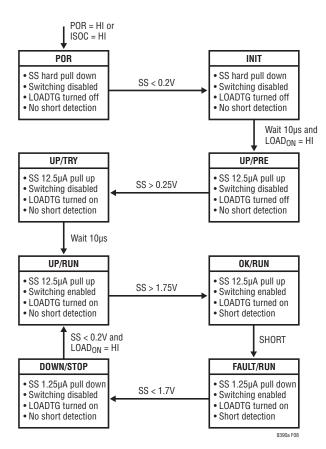
Figure 8. Start-Up and Fault Sequence
