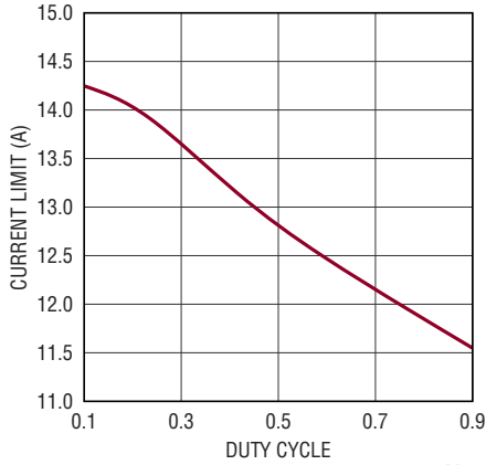
Top FET Current Limit vs Duty Cycle
