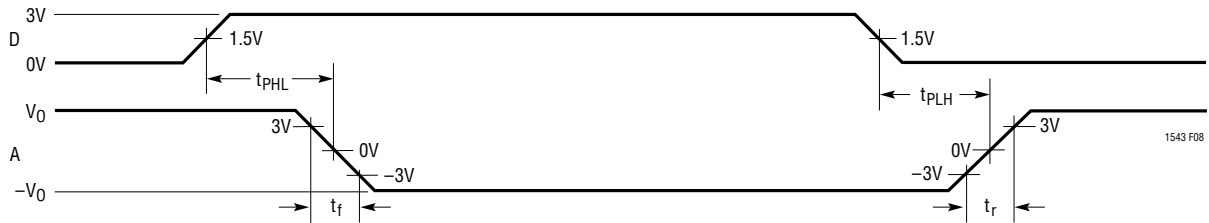
Figure 8. V.10, V.28 Driver Propagation Delays
