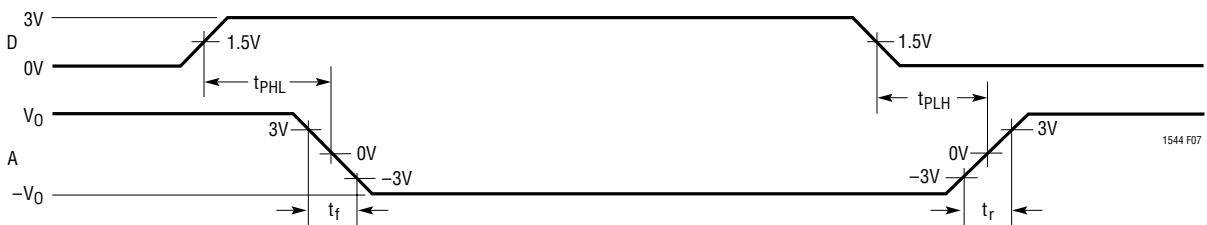
Figure 7. V.10, V.28 Driver Propagation Delays
