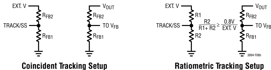
Figure 8(b): Setup for Ratiometric and Coincident Tracking
