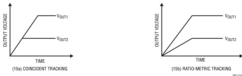
Figure 15. Two Different Methods of Output Voltage Tracking
