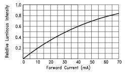
Fig.4 Relative Luminous Intensity v.s Forward Current
