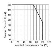
Fig.3 Forward Current v.s Ambient Temperature
