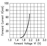
Fig.2 Forward Current v.s Forward Voltage
