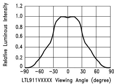
Fig.5-1 Relative Luminous Intensity v.s Off Axis Angle
