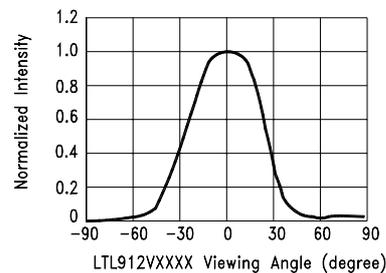
Fig.5-2 Relative Luminous Intensity v.s Off Axis Angle
