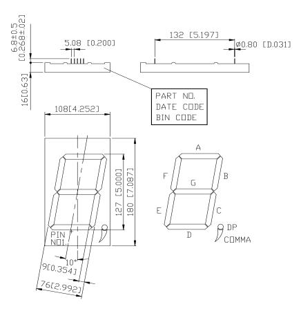
NOTES: All dimensions are in millimeters. Tolerance is  $\pm$  0.25-mm (0.01") unless otherwise noted.
