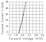
Fig.2 FORWARD CURRENT VS. FORWARD VOLTAGE
