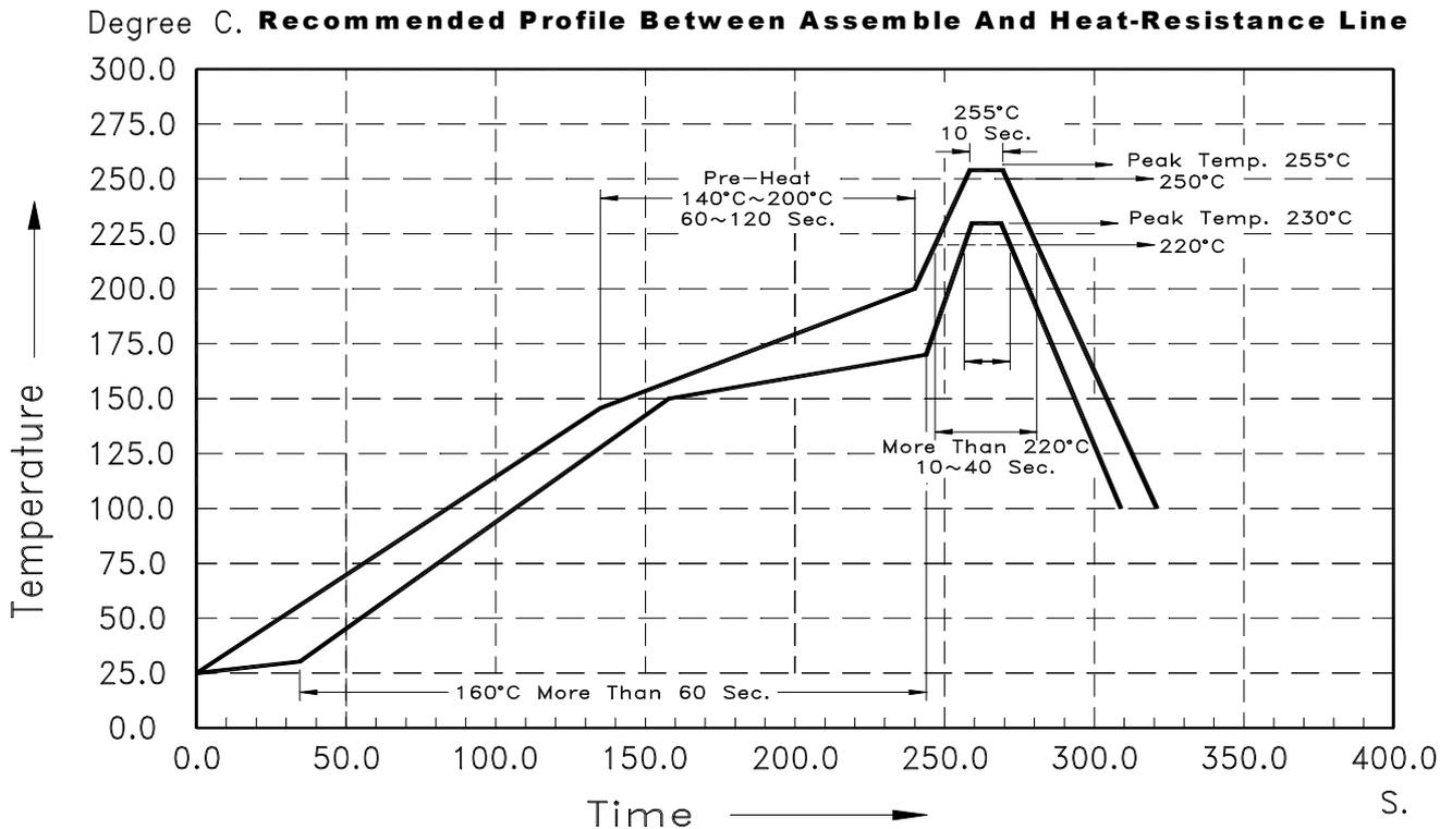
The Profile is available that must to use SnAg<sub>(x=3.3~3.8)</sub> Cu<sub>(y=0.2~0.7)</sub> solder paste
