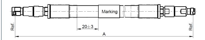
All dimensions are in mm; tolerances: ± 3mm for A ≤ 300 mm; ± 1% for A > 300 mm
