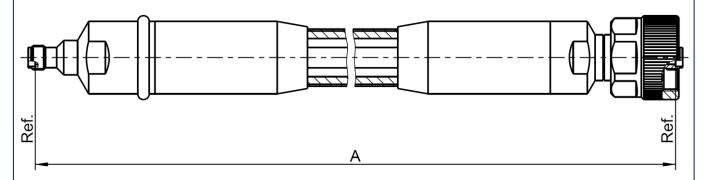
All dimensions are in mm; tolerances: ± 3mm for A ≤ 300 mm; ± 1% for A > 300 mm
